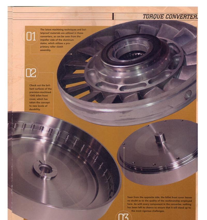
torque with a stall torque ratio of around 1.94:1-depending on the design-PI converters increase that ratio to something around 2.30:1, for an increase of about 18.5 percent. Considering the substantial horsepower figures produced by today's enhanced diesel engines, this is quite an improvement.
