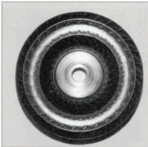
All impeller fins are furnace-brazed for strength and rigidity. The angles of the impeller fins are also important in determining the stall speed.
