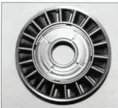
Notice the race on the inside of the stator. It is manufactured from a special alloy that is much harder than the stock piece to resist brinnelling (see photo below). The stator is used to reverse the direction of fluid coming out of the turbine. This gives the converter its torque multiplication capability.
