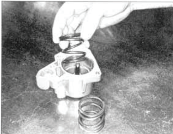
12 The accumulator piston spring is removed and replaced with a stiffer spring. The accumulator valve spring installed in the valve body works in conjunction with the new, stiffer 1-2 accumulator piston spring for firmer shifts.
